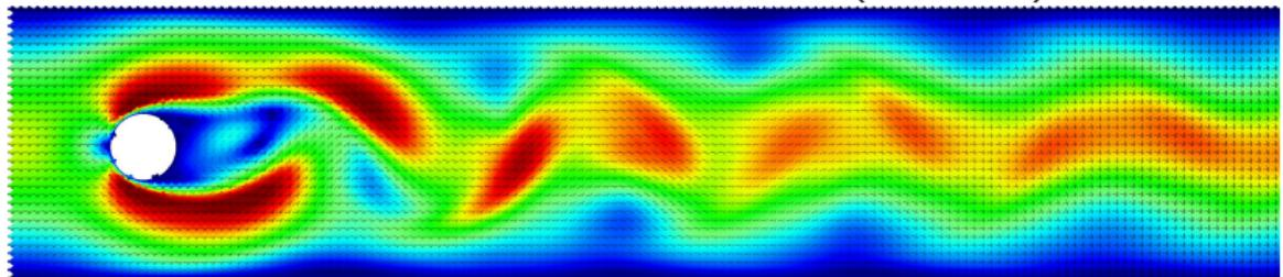
3D laminar flow around a cylinder ( $Re=100$ ):
