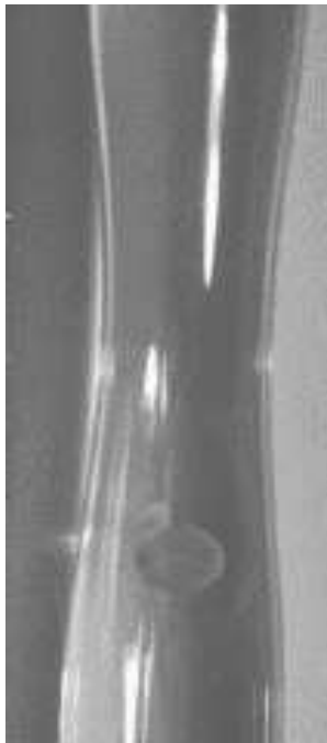
FIG. 5.1. Measuring cell with levitated toluol droplet in downward flowing water
