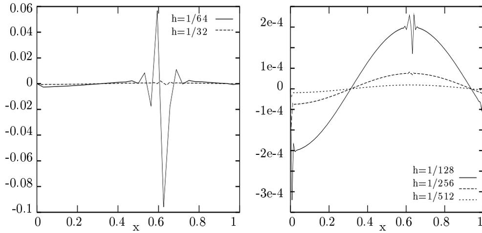
FIG. 5.3. Error in FE solutions in the Experiment Ib,  $\nu = 10^{-6}$ ,  $y = 0.5$
