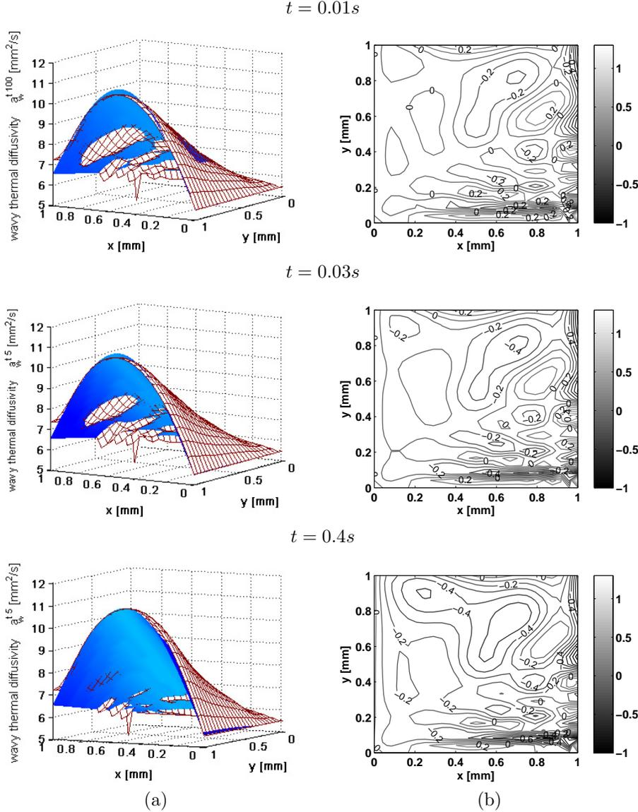
FIG. 4. (a) Estimated (meshed surface) and exact (shaded surface) wavy thermal diffusivities  $a_w^t$ , (b) deviation between exact and estimated wavy thermal diffusivities  $a_w^t$  at different times.
