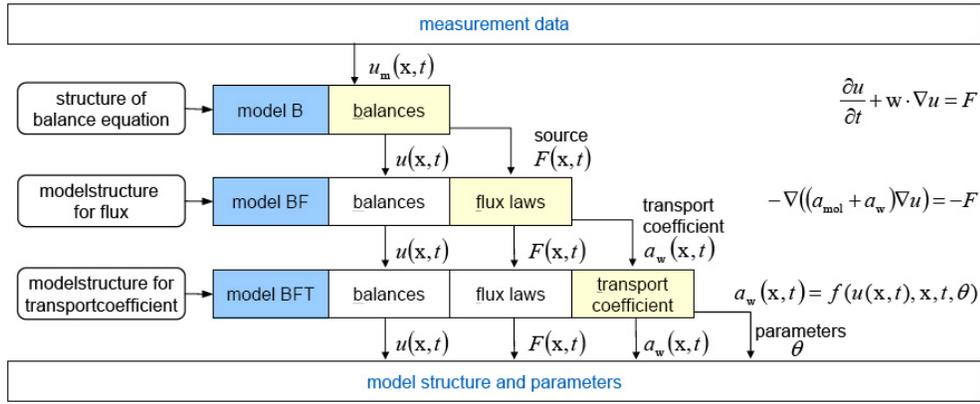
FIG. 1. Incremental modeling and identification of transport phenomena.
