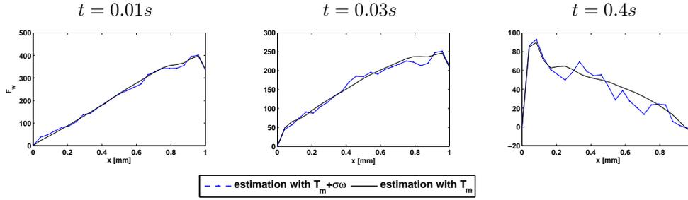
FIG. 11. Estimated source  $F_w$  with unperturbed measurements for  $n_{opt} = 200$  and perturbed measurements for  $\sigma = 0.1$  for ( $n_{opt} = 100$ ) at different times.
