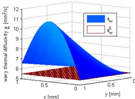
FIG. 1. Initial approximation for the wavy thermal diffusivity  $a_w^t$  at  $t = 0.01s$  and constant  $z = 0.5 mm$ .
