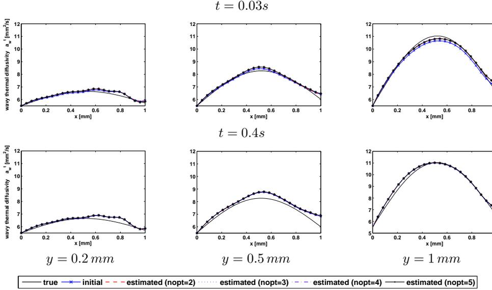
FIG. 7. Estimated wavy thermal diffusivity  $a_w^t$  at different outer optimization iterations  $nopt$ , two different times, three different  $y$  and constant  $z = 0.5$  mm.
