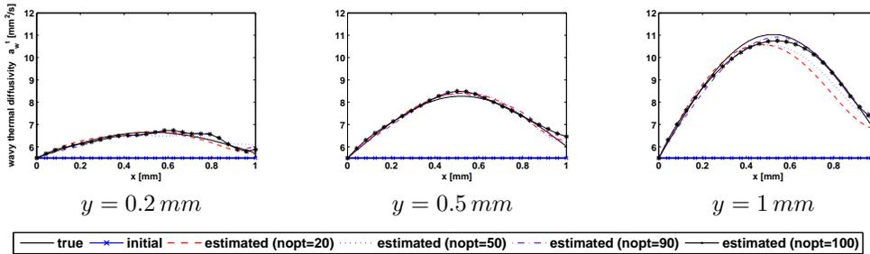
FIG. 6. Estimated wavy thermal diffusivity  $a_w^t$  at different Newton iterations  $nopt$ , time  $t = 0.01s$ , different  $y$  and constant  $z = 0.5 mm$ .
