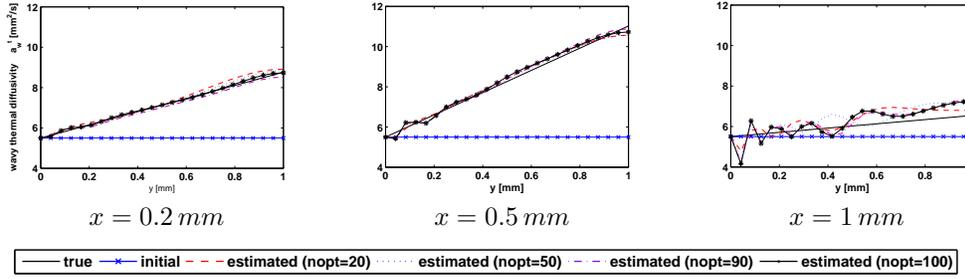
FIG. 5. Estimated wavy thermal diffusivity  $a_w^t$  at different Newton iterations  $nopt$ , time  $t = 0.01s$ , different  $x$  and constant  $z = 0.5 mm$ .
