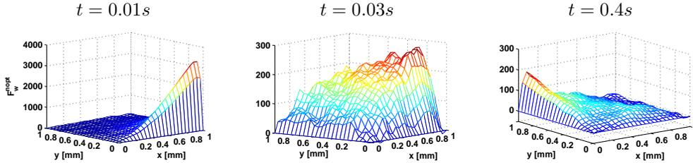
FIG. 10. Estimated source  $F_w$  at different times for constant  $z = 0.5\text{ mm}$  with perturbed measurements ( $\sigma = 0.1$ ) for  $n_{opt} = 100$ .
