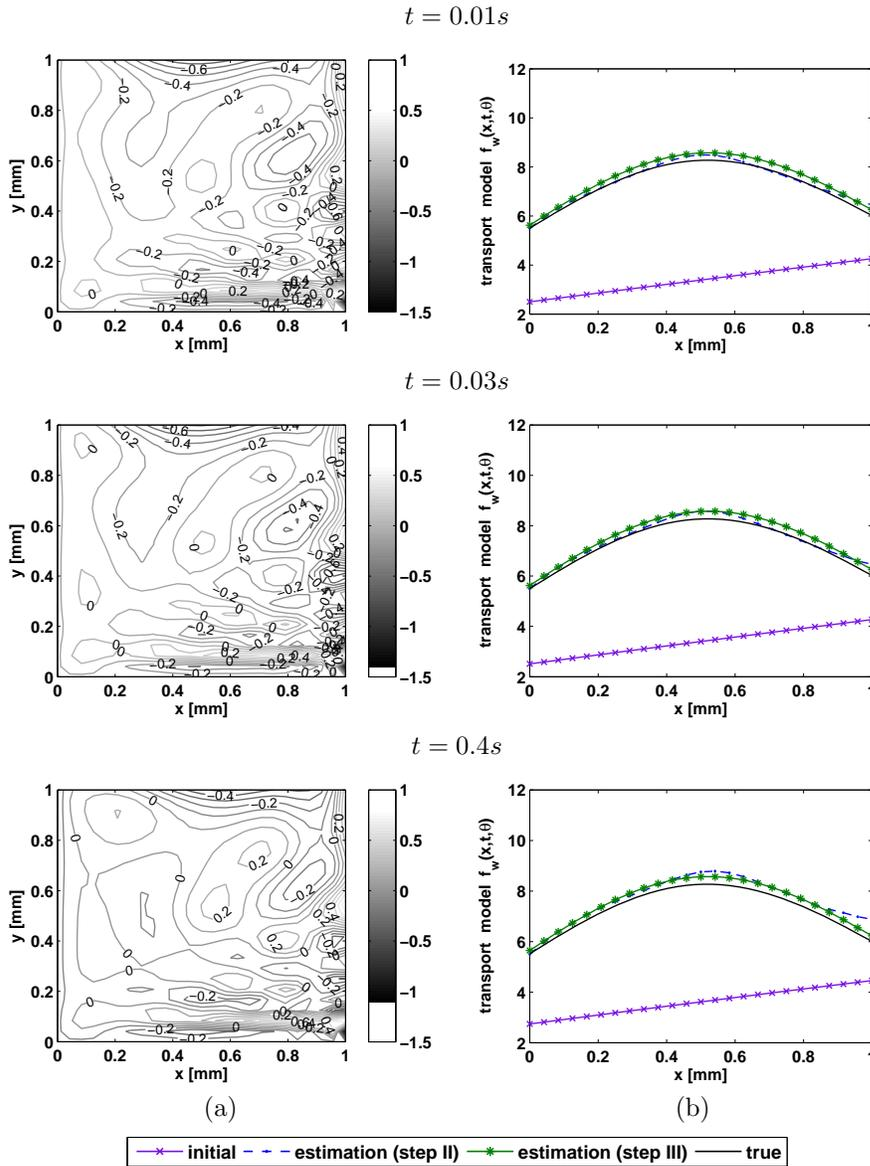
FIG. 8. (a) Deviation between the wavy thermal diffusivity estimated in the second step and the model  $f_w$  estimated in the third step of the incremental approach (b) "true" wavy thermal diffusivity, estimated wavy thermal diffusivity  $a_w^t$  in the second step and estimated model  $f_w$  in the third step of the incremental approach at different times for constant  $y = 0.5 \text{ mm}$  and  $z = 0.5 \text{ mm}$
