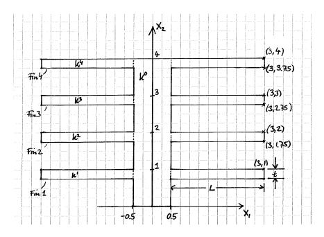
Figure 1: Reference geomtry of thermal fin.
