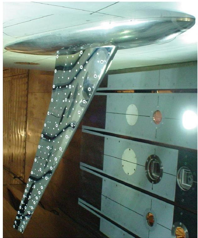
Figure 1: Manufactured model mounted ETW.
